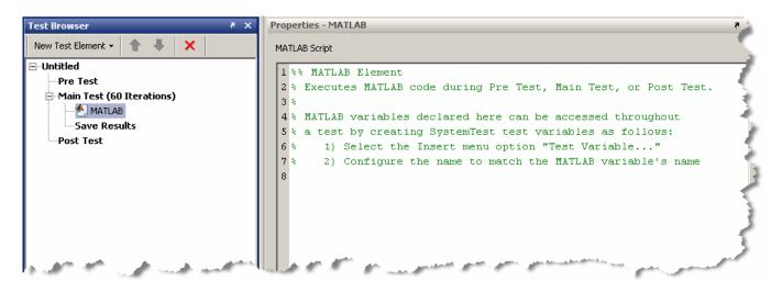
**3** In the **Properties** pane, type the following M-code in the MATLAB Script edit box. This MATLAB code calculates a value for Y that is dependent on the test vector signal.
