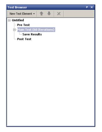
2 Specify the element you want to add to the test section. For this example, click the **New Test Element** button and select **MATLAB**. SystemTest adds a MATLAB element to the Main Test section of your test and opens the MATLAB element property page in the **Properties** pane of the SystemTest desktop.
