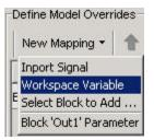
2 Select the workspace variable you want to override. Click the **Simulink Data** field of this row to see all available base workspace variables and Simulink model workspace variables. For the Inverted Pendulum example, select **masspend**.
