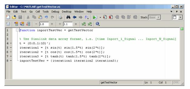
Once this function is saved as GETTESTVECTOR, you can create a SystemTest test vector whose expression is set to GETTESTVECTOR. This will create a 1-by-3 test vector cell array within SystemTest, where each entry in the cell array represents the time and signal data for the three Inport blocks.
