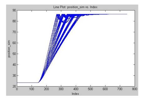
This output shows that the test results group in small clusters. You can use a constraint to see which of the test vectors cause this clustering.
