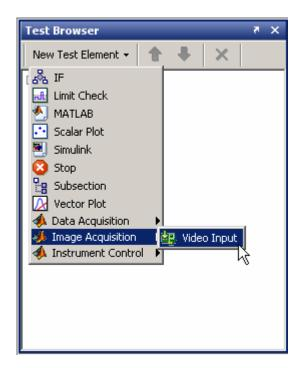
SystemTest adds the Video Input element to the Main Test section of the test and displays the **Properties** pane for the Video Input element. (You can also add elements to the Pre Test or Post Test sections of a test but this example does not require it.)
