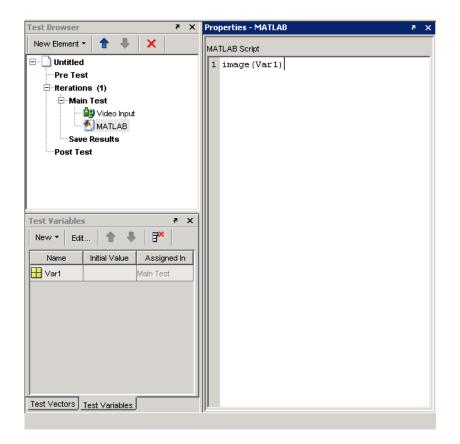
This completes this example test illustrating how to incorporate image data into SystemTest. In a real testing application, you can define test vectors that determine the number of iterations of your test that SystemTest performs. You can also compare test variables against defined limits in the Limit Check element and specify pass/fail criteria.
